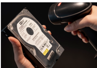
Scans serial numbers of hard disks before erasure
